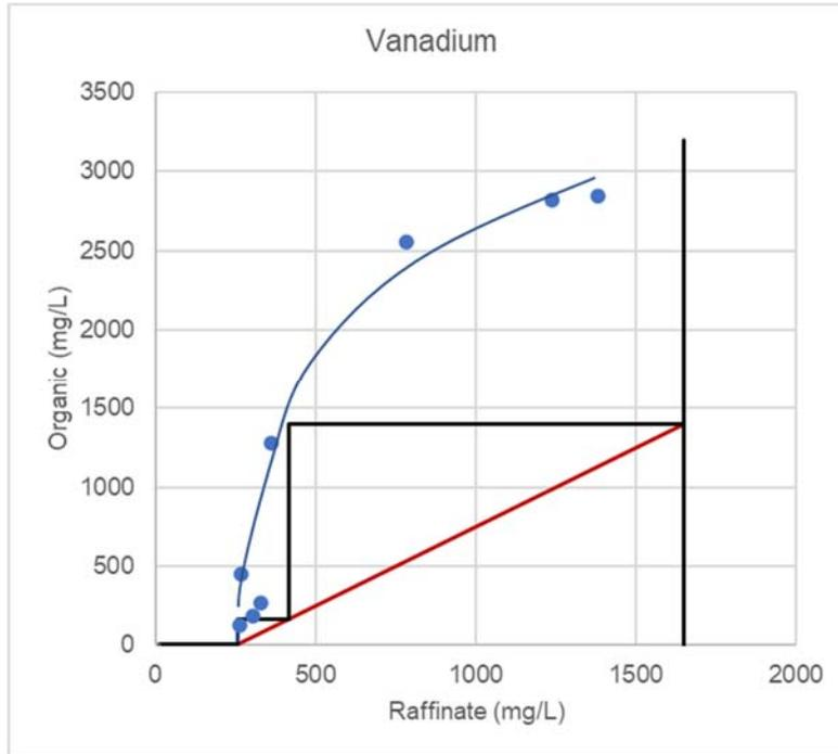
Figure prepared by SGS Minerals, 2019. 1% Alamine 336 in Aromatic 150ND, washed 2x with 20 g/L H<sub>2</sub>SO<sub>4</sub> prior to use. T = 45° C and pH 1.5. Aqueous to organic volumetric ratio (A:O ratio) of 10:1, 7:1, 3:1, 1:1, 1:3, 1:7 and 1:10.
